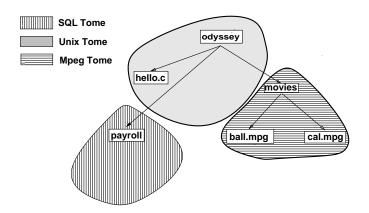
This figure shows a hypothetical Odyssey name space. It has three tomes, each from a different codex. The root tome is from a UNIX file codex. Embedded in it are mount points to an Mpeg tome, with root movies, and an SQL tome, with root payroll. The internal name structure of the Mpeg tome is hierarchical: a directory with two movies, ball.mpg and cal.mpg, is visible. The SQL tome, however, has no internal naming visible at this level.
